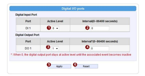
DI: To setup DI, please define the Active level as 0 or 1. If the active level is set as 1, then camera will consider high voltage difference a trigger, which can be used to initiate other events. The event will end when the DI voltage goes back to 0. Interval determines the minimum delay that must pass before the IP device will accept another trigger from DI ( in seconds). 0 means there is no minimum delay limit.
