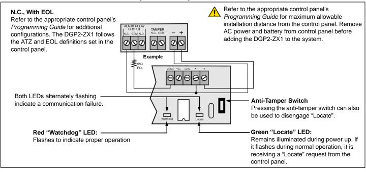
Figure 2: Connecting the Combus
