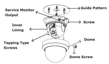
**Note 1**: Use the machine type screws if you are attaching the camera to a pendent mount. Use the tapping type screws for all other surfaces.
