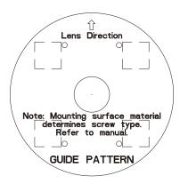
**Mark hole positions:** Secure the metal plate to the ceiling using the appropriate screws.
