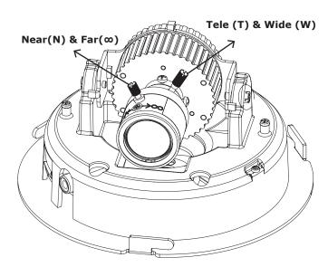
Note 1: Re-tighten the screws after focus adjustments are done.
