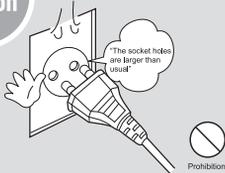
**If the socket holes are larger than normal, do not put the plug.**
