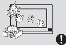
**Avoid direct rays of the sun or heating devices at a time of installation.**
