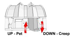
Remove detector assembly as described in Step 1. When selector is UP, Pet Mode; when DOWN, Creep Zone is active and there is no Pet Immunity. Above 2.4m Pet Immune should be OFF (lever down Pet OFF, see installation height note\*.
